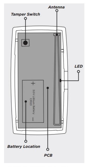
Figure 3: PCB Components
