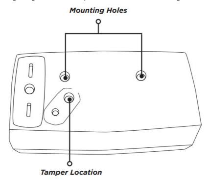
Figure 4: Mounting Holes
