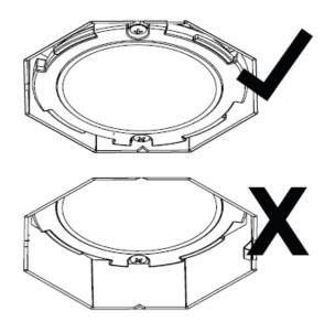
14. Align trim onto the module and turn the trim clockwise until secure.
