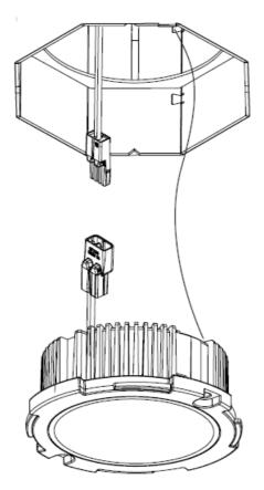
13. Place the module into the junction box, aligning screws with washers to screw holes in the junction box bracket. Screw to the junction box.
