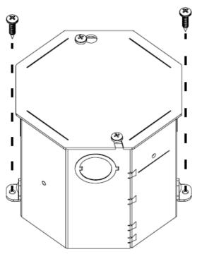
3. Remove screws from the junction box lid and remove the lid.
