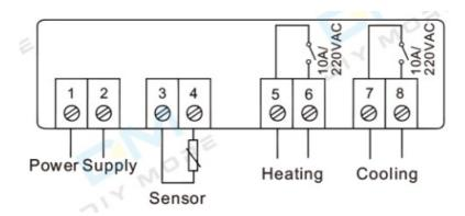
Connection 1: Independent power supply for load
