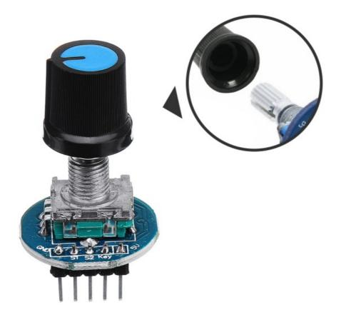
Easy to install and use, no tools required, just put the switch cap onthe switch head and press the switch knob firmly.
