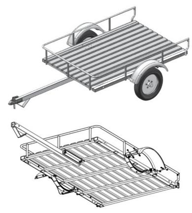
NOTE: The above drawing shows the trailer from below with axle and wheels removed for clarity.
