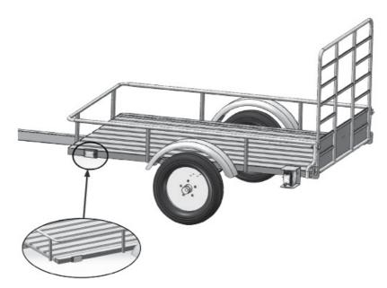
NOTE: Use dialectric grease on each connector for corrosion prevention.
