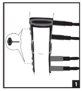
The screws will feel loose when a neutral brace position is achieved. Continue to adjust the screws to achieve the desired load.
