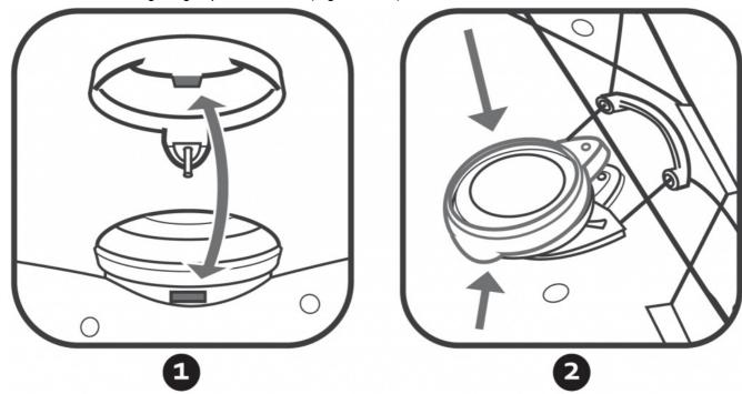
Warning: If the Boa® Reel is in the up position, the Locking Ring will not engage properly.
