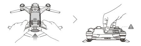
Hold the rear arms of the aircraft and push the Intelligent Flight Battery in place all the way to the end. Push and pull the battery to check that it is securely clamped.
