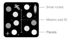
Small rocket: This represents the positive direction of the x-axis in the mission pad coordinate system.
