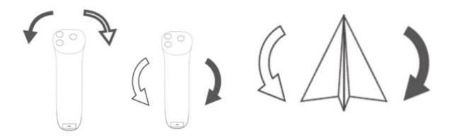
Tilt the motion controller up and down to control the tilt of the gimbal.
