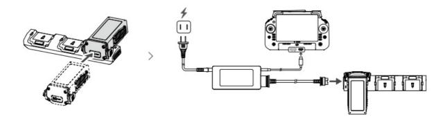
Charge the remote controller to activate the internal battery before using for the first time.
