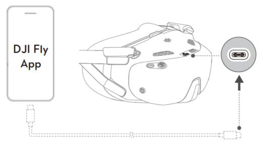
• Run DJI Fly on the mobile device and follow the prompts to activate the DJI devices. Follow the prompts in the goggles if unable to connect to the mobile device.
