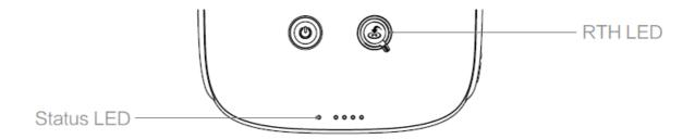
The Status LED reflects connection status between the Ground System and Air System. The RTH LED shows the Return to Home status of the aircraft. The table below contains details of these indicators.
