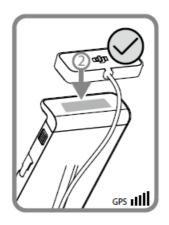
3. Fasten the cable and the mobile device holder to prevent it from dangling with the Velcro strap. Ensure that the cable hangs down beneath the remote controller alongside one side of the antennas. DO NOT place the cable through the middle of the antennas.
