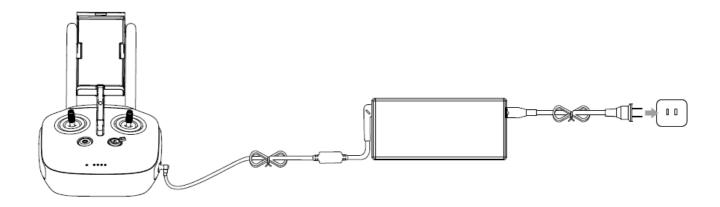
The status LED will turn off when charging is complete. It takes about four hours to fully charge the Ground System.
