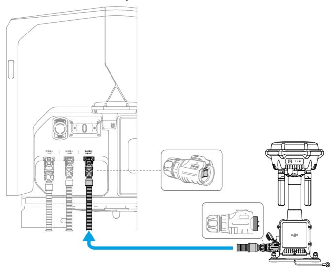
• When connecting to a PoE power adapter, follow the T568B wiring standards to make the Ethernet connector. Make sure that the PoE power supply is not less than 30 W.
