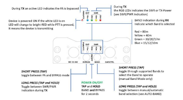
The correct Band must be selected, otherwise the PA will not transmit
