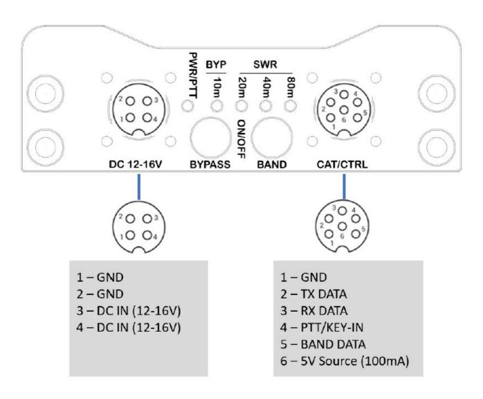
there is no reverse polarity protection, incorrect wiring will destroy the device.
