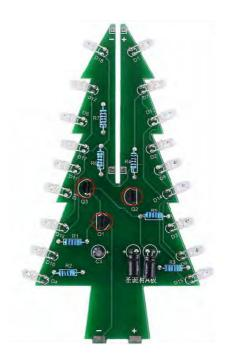
Step 6: Install PCB-B. Install 3pcs 100ohm Metal Film Resistor on R2, R4, and R6.
