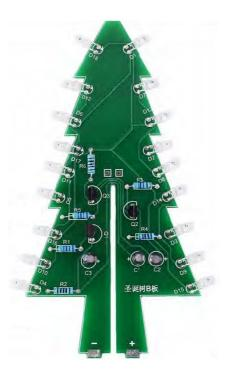
**Step 11:** Test. Connect 4.5V-5V to PCB-A and PCB-B separately. Preliminary welding success if LEDs are blinking automatically.
