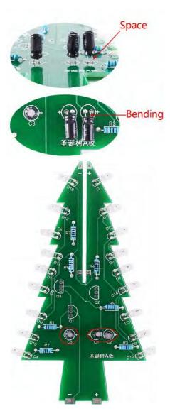
**Step 5:** Install 3pcs TO-92 S9014 Transistor at Q1,Q2,Q3.It is better to bend S9014's pin so that 2pcs PCB-A and PCB-B can better splicing.OK, PCB-A has been installed and completed.
