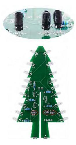
**Step 10:** Install 3pcs TO-92 S9014 Transistor at Q1,Q2,Q3.It is better to bend S9014's pin so that 2pcs PCB-A and PCB-B can better splicing.OK, PCB-B has been installed and completed.
