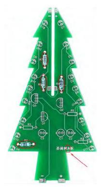
Step 2: Install 3pcs 4.7K Metal Film Resistor on R1, R3, R5.
