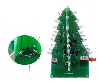
Step 16: Install the top LED Note the positive and negative of LED. At this point, The installation is complete!!
