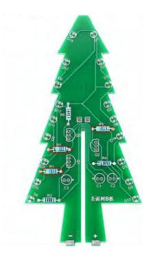
**Step 8:** Install 18pcs 3mm RGB LED at D1-D18.Pay attention to distinguish the positive and negative poles of LED and the Longer pin are positive pole. Control distance between PCB edge and LED head.
