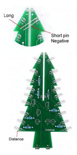
**Step 4:** Install 3pcs 47uF 16V Electrolytic Capacitor at C1,C2,C3.Pay attention to distinguishing the positive and negative poles and the Longer pin are positive poles. A 2~3mm spacing is reserved between the capacitor and the PCB to facilitate the bending of the capacitor for subsequent installation.
