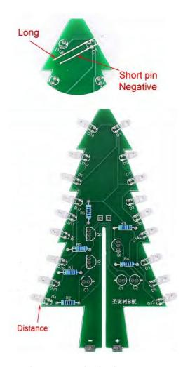
**Step 9:** Install 3pcs 47uF 16V Electrolytic Capacitor at C1,C2,C3.Pay attention to distinguishing the positive and negative poles and the Longer pin are positive pole.A 2~3mm spacing is reserved between the capacitor and the PCB to facilitate the bending of the capacitor for subsequent installation.
