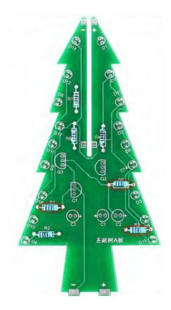
**Step 3:** Install 18pcs 3mm RGB LED at D1-D18.Pay attention to distinguishing the positive and negative poles of LED and the Longer pin are positive pole. Control distance between PCB edge and LED head.
