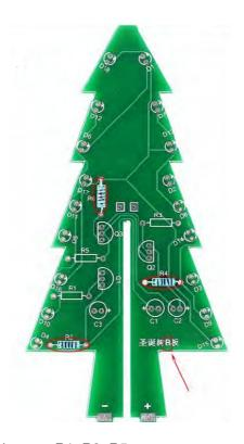
Step 7: Install 3pcs 4.7K Metal Film Resistor on R1, R3, R5.
