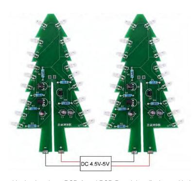
Step 12: Align the two positioning heads on PCB-A and PCB-B and then fix them with tin.
