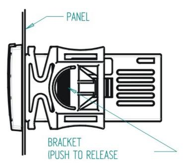
Instrument XR70CH shall be mounted on vertical panel, in a 29×71 mm hole, and fixed using the special bracket supplied.
