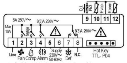
**NOTE:** The compressor relay is 8(3)A or 16(6)A according to the model.
