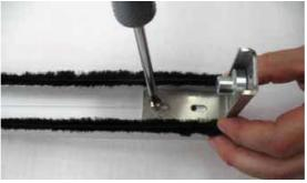
22. Fasten detail [20] to the lower portion of profile 3809, as shown in the diagram.
