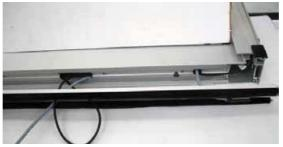
15. Feed the cable through the upper portion of the wing and make it to come out in correspondence to the photocell cable, as shown in the diagram.
