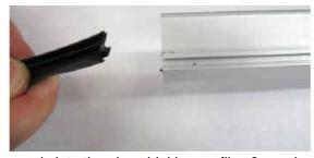
27. With PAM45M profiles, insert the seals into the glass-bloking profiles 8, as shown in the diagram.
