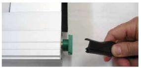
24. Insert seal 3838 into profile 3831, as shown in the dia- gram, and block it to prevent it from sliding
