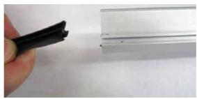
28. With PAM45M profiles, insert the seals into the glass-blo- king profiles [8], as shown in the diagram.
