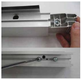
4. Join the vertical profiles with the horizontal profiles and fa- sten them as shown in the diagram.
