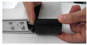
19. Insert detail [6] into profile 3820 near detail [3], as shown in the diagram
