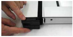
20. Insert detail [7) into profile 3820, as shown in the dia- gram.
