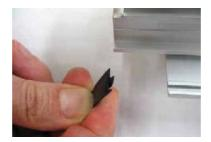
1. Insert the seal 3839 into the PAM45M profiles 3800, 3808 and 3813 or else the PAM45L profiles 3599, 3821 and 3822, as shown in the diagram.
