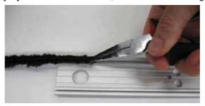
13. Insert the brush SPAZ4811 into profiles 3924 and 3809, as shown in the diagram, and block it to prevent it from sliding.
