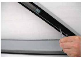
15. 4.15 Fasten detail [3] to profile 3820, as shown in the diagram.
