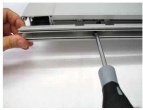
5. Fasten profile 3805 to the lower portion of the wing, as shown in the diagram.
