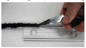
10. Insert the brush SPAZ4811 into profiles 3924 and 3820, as shown in the diagram, and block it to prevent it from sliding.
