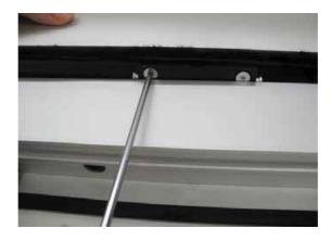
**Note:** during the installation of the fixture. in order to obtain the proper breakaway strength for the mobile wing, use the lateral screws to adjust detail (5], as shown in the diagram 2.
