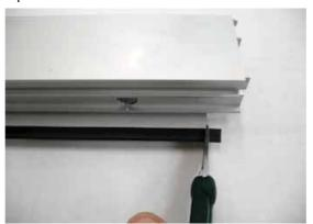
3. Insert detail [1] into the PAM45M profiles 3800 and 3813 or else the PAM45L profiles 3599 and 3822, and fasten it as shown in the diagram.
