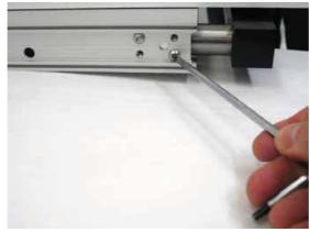
9. Fasten detail [3] by tightening the eight fastening screws, as shown in the diagram.
