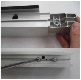
3. Insert detail [1] into the PAM45M profiles 3800 and 3813 or else the PAM45L profiles 3599 and 3822, and fasten it as shown in the diagram.
