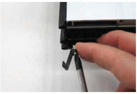
22. Attach the supplied hook to the lower part of the wing, as shown in the diagram, in order to prevent seal 3837 from sliding.
