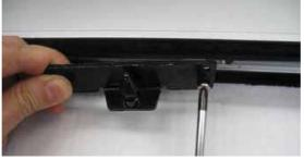
13. Trim the brush SPAZ4811 where it connects with detail (5], as shown in the diagram. Note: Be sure to take note of the wing's opening direction
