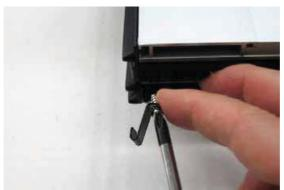
22. Attach the supplied hook to the lower part of the wing, as shown in the diagram, in order to prevent seal 3837 from sliding.
