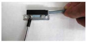
12. Attach the magnetic limit switch [15] to its relative bracket, as shown in the diagram
