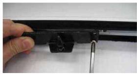
12. Fasten detail [4] to profile 3924, as shown in the diagram.
