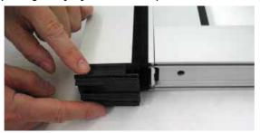
21. Insert detail [7] into profile 3820, as shown in the diagram.
