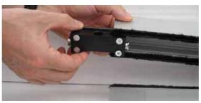
17. Insert detail [5] into profile 3820, as shown in the diagram.
