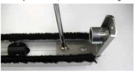
23. Fasten detail [21] to the upper portion of profile 3809, as shown in the diagram.
