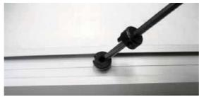
20. Fasten the expanders [18] to the perimeter profiles 3809, as shown in the diagram, using the appropriate 6 mm Allen key.
