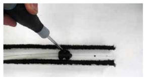
21. Fasten detail [19] to profile 3809, as shown in the diagram.
