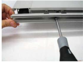
5. Fasten profile 3805 to the lower portion of the wing, as shown in the diagram.
