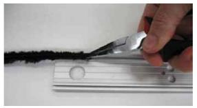
10. Insert the brush SPAZ4811 into profiles 3924 and 3820, as shown in the diagram, and block it to prevent it from sliding
