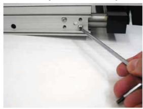
9. Fasten detail [3] by tightening the eight fastening screws, as shown in the diagram.
