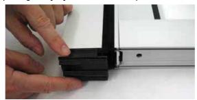
21. Insert detail [7] into profile 3820, as shown in the diagram.
