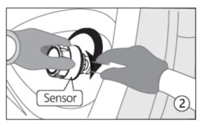
2. Install the sensor onto the tire valve clockwise.
