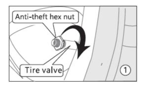
1. Install the anti-theft hex nut onto the tire valve.
