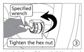
3. Tighten the anti-theft hex nut counter clockwise until the nut is tightened against the sensor.
