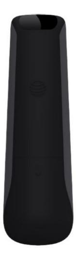
RC83V remote works in IR and Bluetooth interface. The remote uses Bluetooth 2-way communication to C71KW. Bluetooth eliminates the need for the remote and the paired devices to be in line of sight to each other. Voice Recognition is available in the RC83V Remote. Voice search will only work when the remote is paired to the C71KW.
