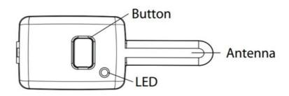
The Control Center, typically located on the upper part of the front windshield receives commands from your system. It consists of:
