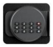
• If the password is incorrectly entered 3 consecutive times, the yellow indicator will blink continuously with an alarm sound.
