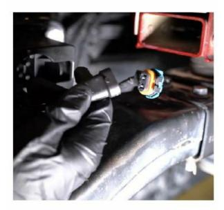
10. If you purchased backlit SS3 pods, connect the backlight power wire to a fused 12V source to trigger the backlight feature (i.e. parking light or sidemarker); T-Taps are included for this purpose. Check local laws and regulations for on-road use of backlight feature.
