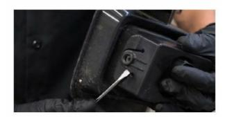
**NOTE**: You may need to loosen the two 15mm bolts on the crash bar to give yourself enough room to remove the fog light bezel.
