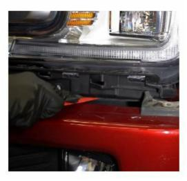
4. Using a plastic trim removal tool, loosen the upper bumper piece. Repeat the steps on the other side of the vehicle to remove the upper bumper piece from the vehicle.
