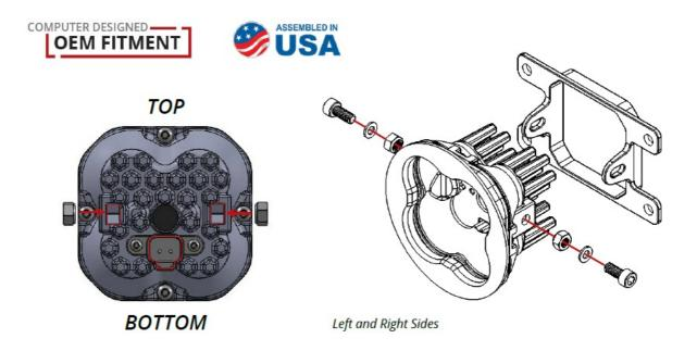
Install the supplied nuts into the pod housing with the nylon facing inward. Attach the bracket to the pod using
