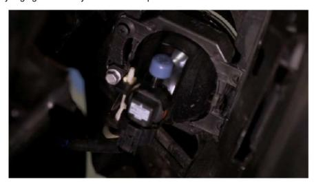
3. Disconnect the fog light connector from the vehicle wiring harness. Remove the factory fog light housing. The factory hardware will be reused.
