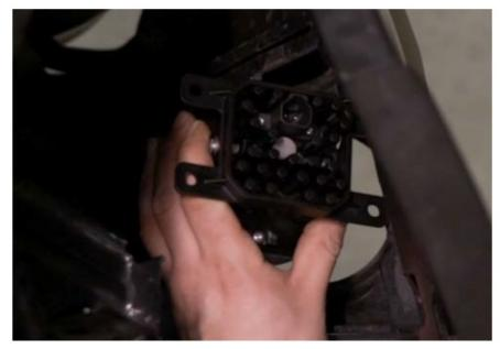
5. Use the included wire adapters to connect the pod to the vehicle wiring harness. Test function. If the light does not turn on, try flipping the connector 180°. If you purchased backlit SS3 pods, connect the backlight power wire to a fused 12V source to trigger the backlight feature (i.e. parking light or sidemarker); T-Taps are included for this purpose. Check local laws and regulations for on-road use of backlight feature
