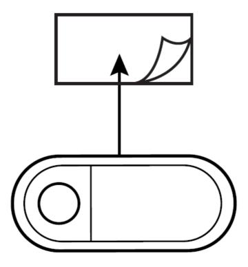
**NOTE:** If you mount your pushbutton on a surface made of uPVC (polyvinyl chloride) or metal, please note that the transmission range will be reduced.
