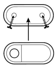
1. Open the transmitter using a flat screwdriver and separate the front and back sections. Then, secure the rear section at an appropriate height on the wall using the two screws provided.
