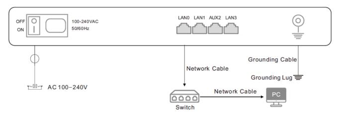
• Connect FXS port with Telephone line, and connect FXO port with PSTN line.
