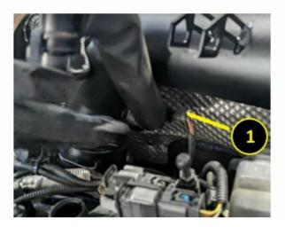
25. Connect lines (1) & (2) to Dinan pipe. Dinan pipe must audibly engage with turbo inlet. Tighten screw (3) to 6 ft-lbs. Connect line (4) to cylinder head cover. Line (4) must audibly engage.
