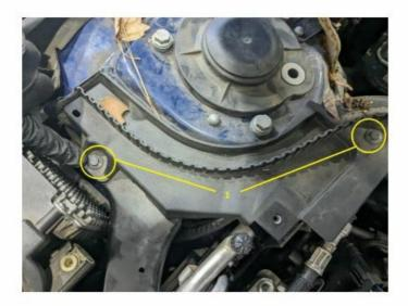
14. Unscrew the 3 screws and unclip fuel line from holder.
