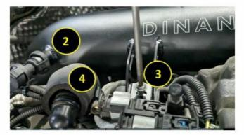
26. First connect the flex pipe (1) to air box and then to Dinan pipe. Ensure flex section orientation is as shown below. Tighten clamps (2) to 2.2 ft-lbs.
