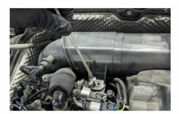
18. Release blow by heater line and disconnect from cylinder head cover.
