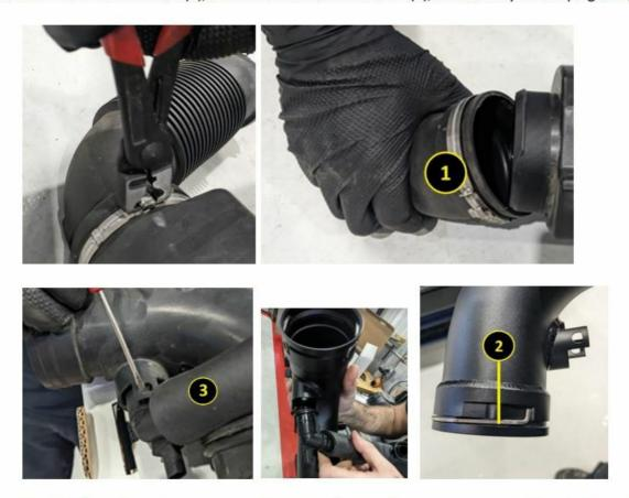
24. Feed in Dinan pipe and attach connector (1) to heating element. Connector (1) must engage audibly.
