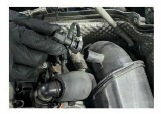
20. Unlock clamp at the turbo inlet.
