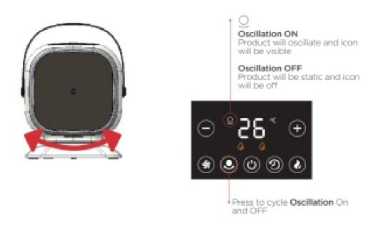
• Oscillation feature provides Heating and Cooling effect across a wide area. This is particularly useful for providing maximum coverage for Heating or Cooling effect quickly and efficiently.
