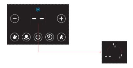
**Default Speed:** This speed is designed to give Medium cooling effect. In cooling mode, when only the fan is running, the segmented display cycles through 3 states to resemble a rotating fan blade
