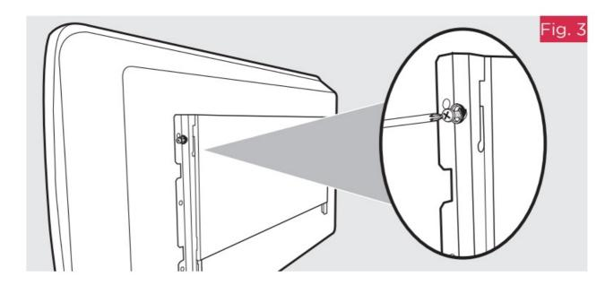
2. Fix the wall bracket securely to the wall through the four screw holes provided referring to dimensions in Fig. 1, Fig. 2.
