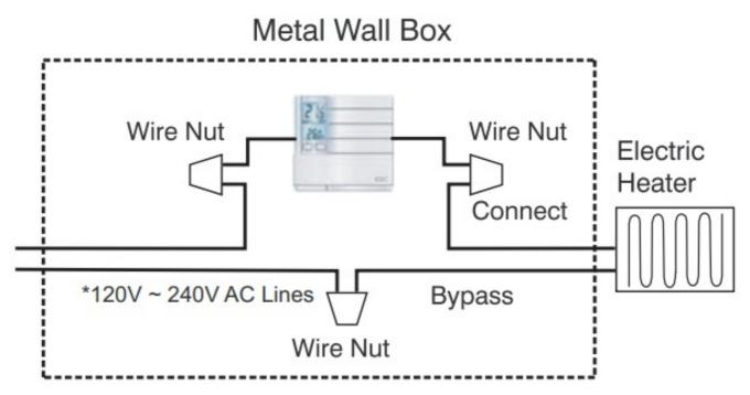
4. Mount the new thermostat onto the wall box using the two screws provided through the mounting holes, and then replace the faceplate. (Place 2 screws in the right side or 2 left holes).
