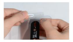
(3) Press the position of the double-sided tape to make it stick firmly
