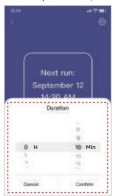
4-3. Manual Watering Set up manual watering duration (1 min- 12h), remaining watering time will be displayed, it will stop automatically when time's up, or shut down manually before time's up.
