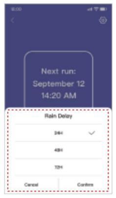
4-2. Rain delay Set up Rain delay duration (24H, 48H, 72H), remaining watering time will be displayed, it will stop automatically when time's up, or shut down manually before time's up.
