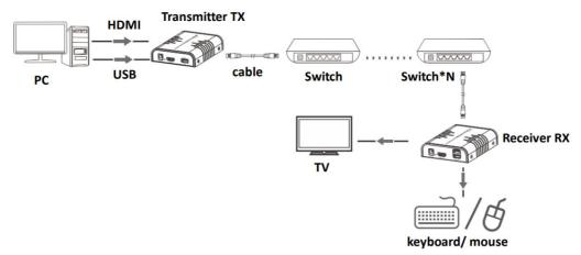
NOTE: Transmission distance depends on the type of network cable, CAT5: 80m, CAT5E: 100m, CAT6: 120m.
