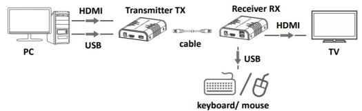
NOTE: Point to multi-point connection via switch is supported too, but under point to multi-point configuration, it is strongly recommended to operate KVM function on one receiver only at the same time.
