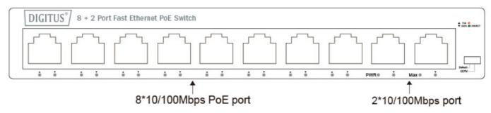
**DIP Switch:** The DIP switch located on the right of the panel.
