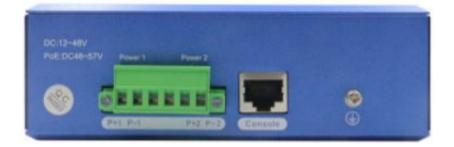
Front panel: the yellow light on RJ45 port is the link light. It is on, when the connection is established and the transmission data is flashing. The green light on RJ45 port is the POE light, which is only on when the switch port supplies power to the downlink PD. Green LED on is for system operation. The power indicator "POW" shows whether the current device is received power in normal.
