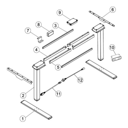
Step 1: Install the supporting beam and the side bracket:
