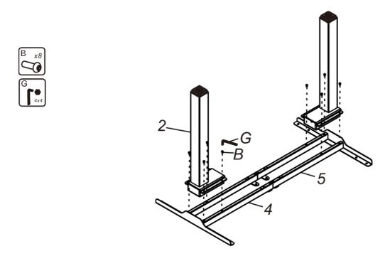
• Using screws (B) to connect the lifting column (2) with the left supporting beam (4) and the right supporting beam (5), and tighten them with the allen key (G)
