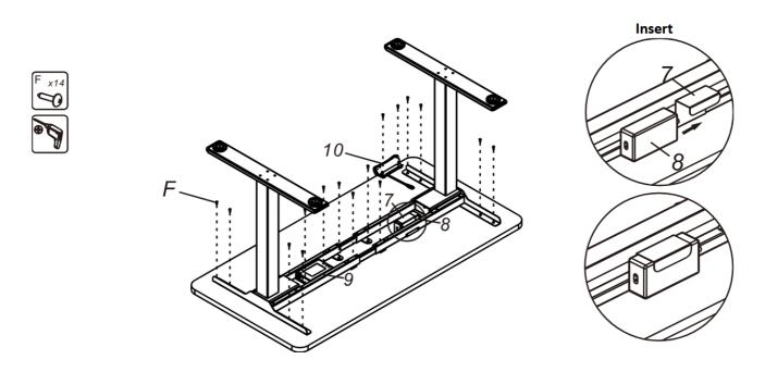
• Fix the tabletop with screws (F), and then to fix the control box (9) on the tabletop with screws (F). The handset (10) is fixed on the tabletop with self- owned screw and insert the adapter into the adapter arm.
