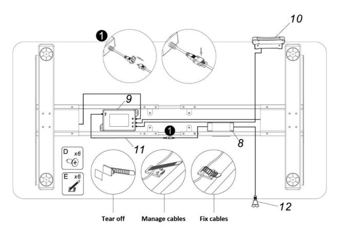
• Fix the cables to the tabletop with cable management (E) and then use screw (D) to fix the cable management (E) to keep the desk cables organized.
