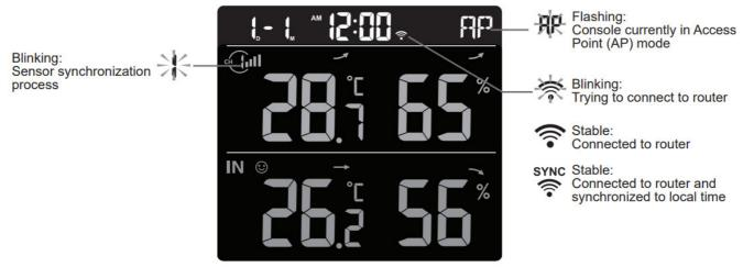
• The wireless sensor will automatically pair up with the console (about 1 minute). Upon successful synchronization, the display will change from "-.-°C -%" to actual reading.
