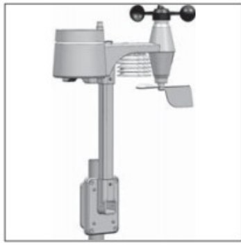
A. Mounting on pole (Pole Diameter 1"~1.3" (25~33mm))
