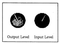
For example, if the INPUT LEVEL is set to the right of center (1 o'clock), set the OUTPUT LEVEL an equal amount to the left of center (11 o'clock).
