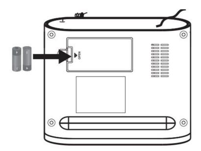
Replace the battery if the device is not used for a prolonged period of time (more than 1 month); Please take the battery out in order to prevent leakage of battery acid.
