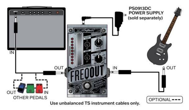
**NOTE**: Since the FreqOut pedal is emulating the interaction between your guitar and an ampliÿer, it is recommended to place it at the beginning of your e°ects chain. This will provide a pure guitar signal and allow the pedal to properly create the feedback harmonics.
