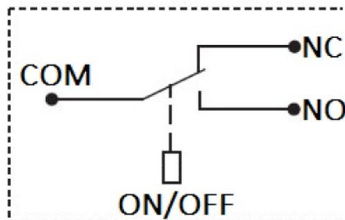
When power is applied, the relay will switch the connection from the Normally Closed NC position, to the Normally Open NO (ie: now closed). You can try this by putting multimeter leads on the common and NO connections, to see when there is a continuity measurement (set the multimeter to beeper) The AA0378 Programmable interval 12V timer module has one relay offering two connections like this, so it is a Double Pole Double Throw relay, or DPDT.
