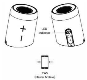
By default, the speaker is connected as one which can be controlled by the main volume buttons on the front of the speaker. If you take off the silicon rubber cover, twist and rotate the speakers to separate them into twin speakers providing you true left and right stereo audio.
