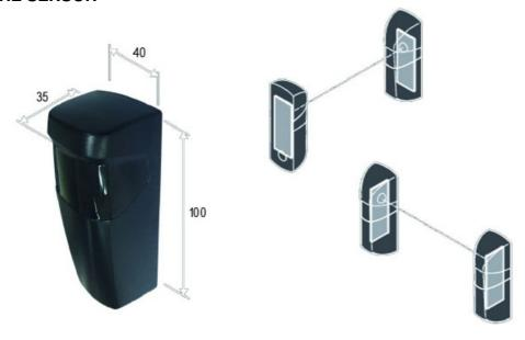
Rotation through 180Ű allows the alignment of the photocells irrespective of the way they are fixed to the base
