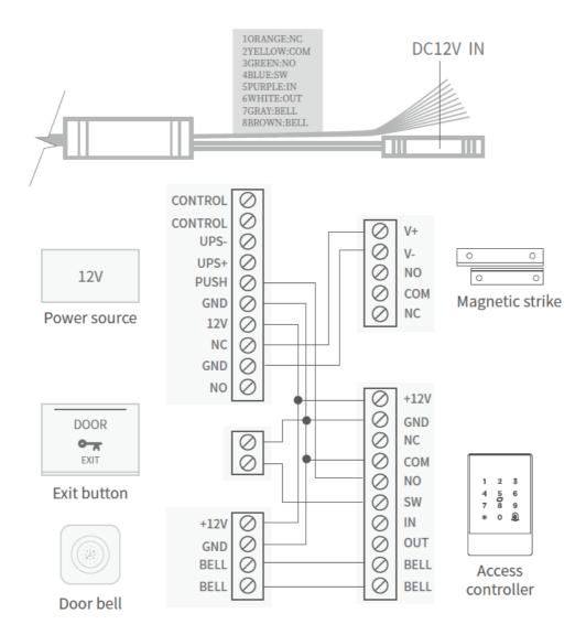
Connect the cable of the access controller to power cable and other ports according to the illustration.
