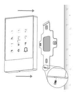
• Fit the access controller into the hook and fix it on the mounting plate with a screw in the bottom.
