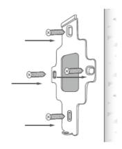
• Fix the mounting plate with 4 screws.
