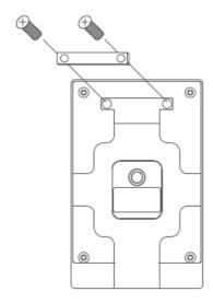
• Fix the hook to the mounting plate with 2 screws.
