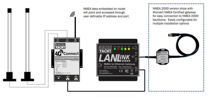
Simple ethernet patch cable connection to router
