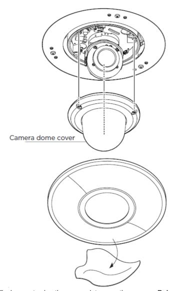
6. Secure the camera to the flush mount using the appropriate mounting screws. Refer to the table below:
