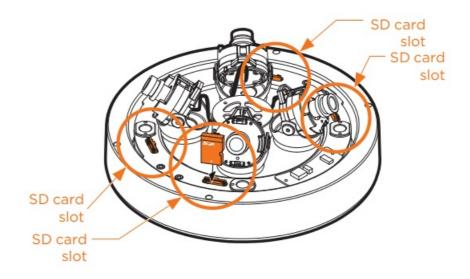
**NOTE:** The camera has four (4) SD card slots, each assigned to a different sensor.
