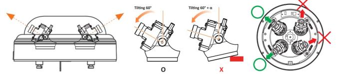
**NOTE:** When installing the camera, align the sensor module's direction as shown in the diagram on the left and fix the dome cover carefully. Image distortion may occur if the modules are not installed correctly.
