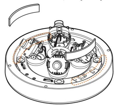
**NOTE:** The camera will generate enough heat to dry moisture during operation. In cases where the camera can experience a moisture issue, keep the moisture absorber in the camera. The moisture absorber has an approximately 6-month life cycle.
