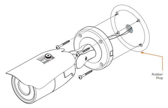
**NOTE:** Remove the rubber plug on the side of the camera's bracket and use the gap as a cable guide to prevent cables from getting caught between the camera and the mounting surface.
