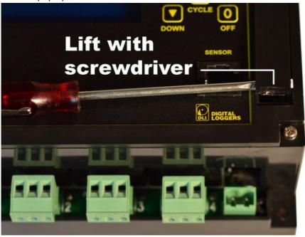
The antenna and/or ADC connector may be attached when the hatch is removed. A three pin connector is provided for ADC input. The upper pin is scaled for 0-100VDC, and the lower pin is 0-10VDC. The center pin is a ground reference bonded to the negative power input.
